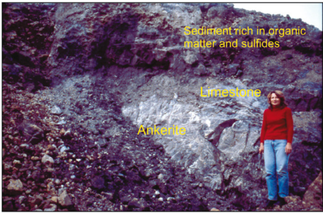
Figure 3. Dark massive siderite and ankerite in contact with dark massive limestones, the Tomašica open-cast mine.
