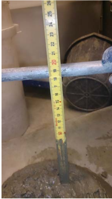
Figur 34. 18 cm synk, betongblanding C.
