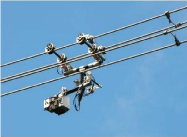
Figure 40: Robot by Expliner [30]
