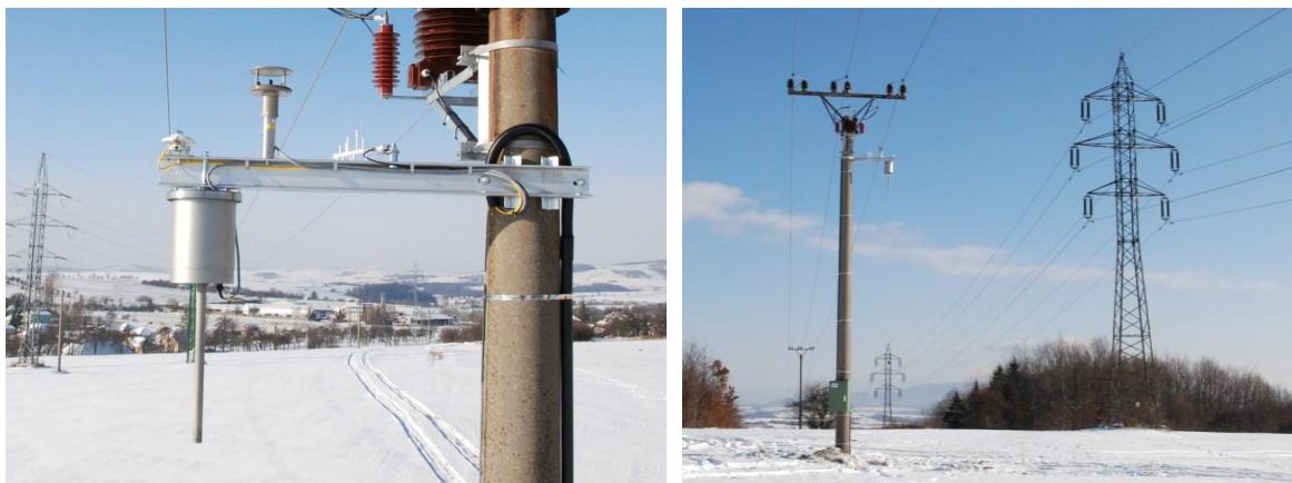
Figure 22: Meteo with Support arm and sensors [20]
