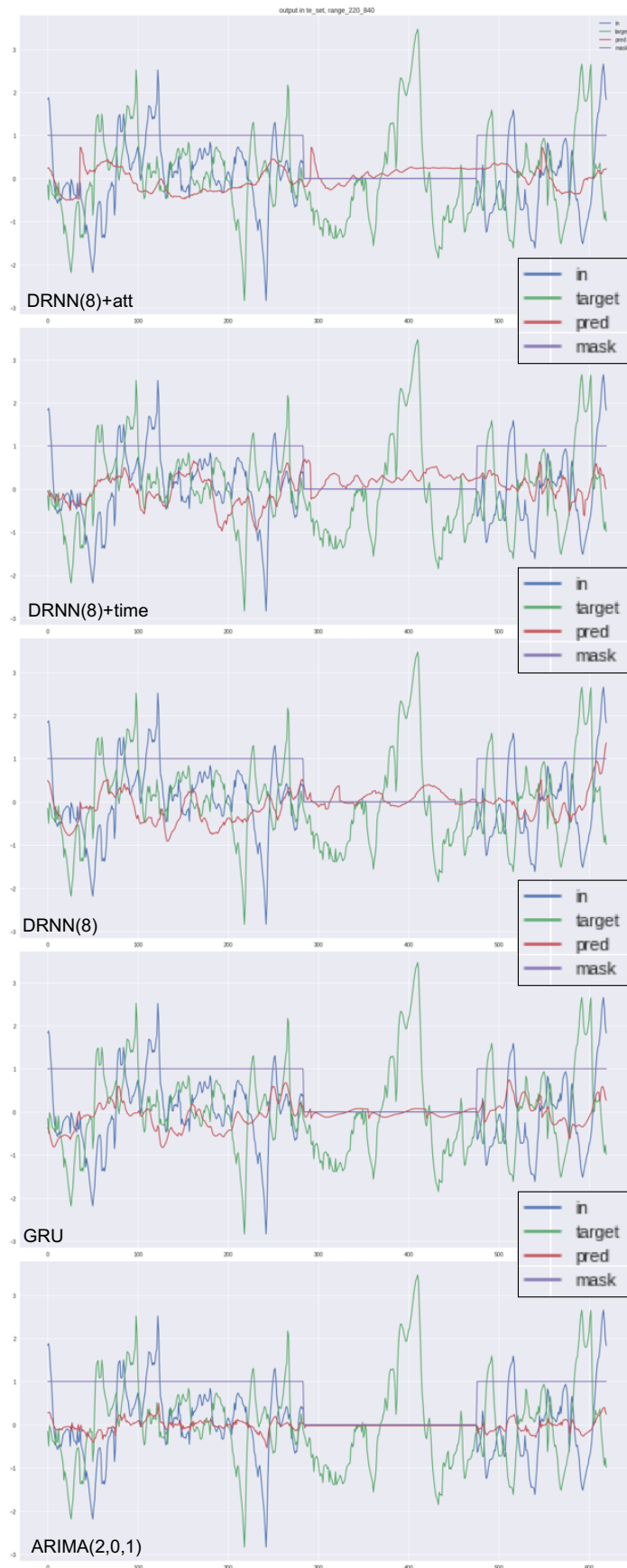
FIGURE 9.9: Forecast plots over a period of time step in test set of GEFCom 2012 after the seasonal differencing at lag 24, depending on the 5 different models. Red line depicts the forecast values while green line depicts the target, that the forecast aims to reach. Blue and violet lines show input and binary mask. From the top, (a) DRNN(8) with modified attention ; (b) DRNN(8) with external RNN with LSTM cell having binary mask as input; (c) DRNN(8). (d) GRU ; (e) ARIMA(2,0,1). Overall, all the models don't make an accurate forecast with GEFCom 2012 set.
