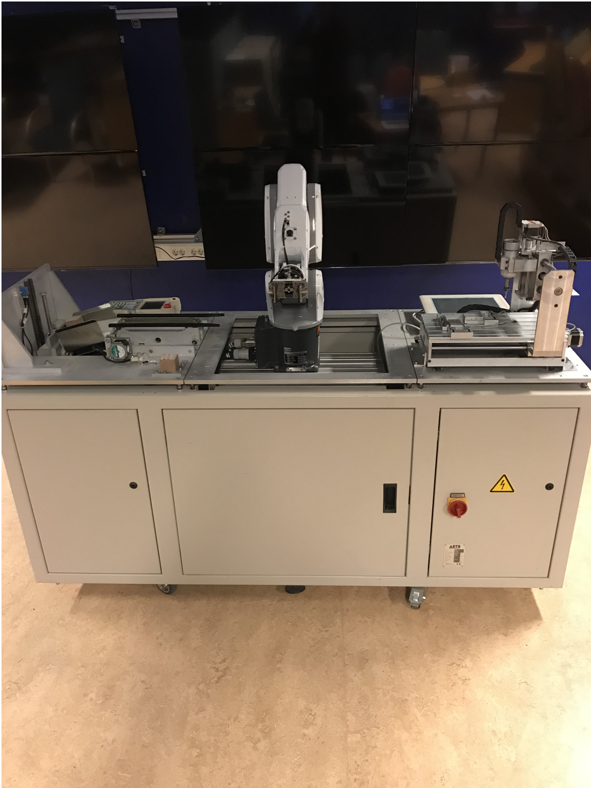
Figure 25: The completed flexible manufacturing system test bench
