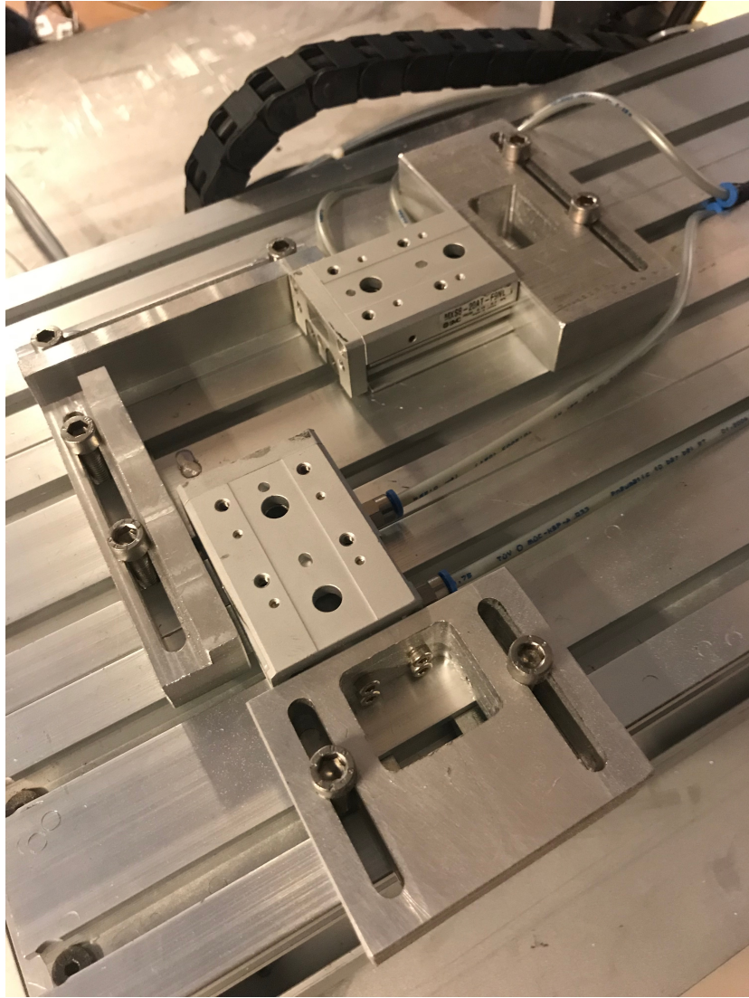
Figure 17: Two pneumatic clamps with holders and two fixed sides with countersunk slots
