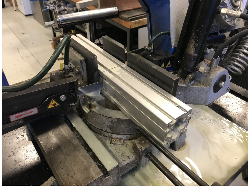
Figure 15: Cutting of the aluminium profiles with a band saw
