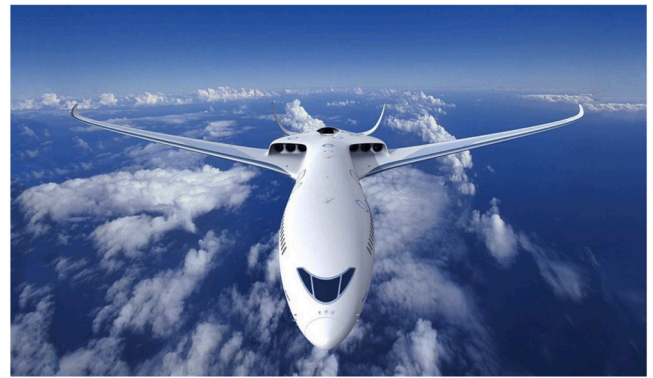
Fig. 15. The Airbus E-thrust aircraft concept utilizes boundary layer ingestion and distributed propulsion [111].
