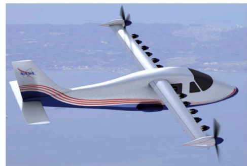
Fig. 12. NASA X-57 Maxwell DEP aircraft [102].
