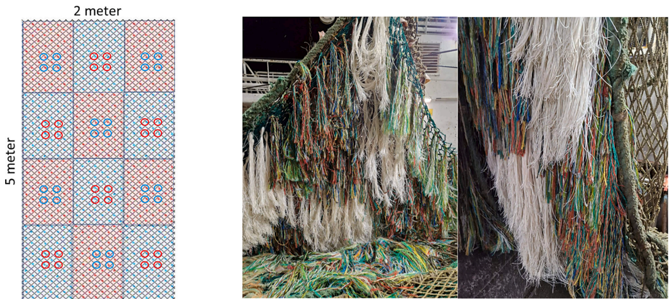
Fig. 4. A trawl codend showing the arrangement of the test (red) and control materials (blue) (left panel). For codend 1, the control material was PE/PP/PET dolly ropes, and the test material was Senbis green rope. For codend 2, the control material was PE/PP/PET dolly ropes, and the test material was PE/PET ropes. The red and blue circles indicate the areas where samples were taken to be length measured and weighed. The photographs to the right show codend 1 with PE/PP/PET dolly rope (blue, red, green fibres) and the Senbis green rope dolly rope (white fibres) before the start of the fishing trials. (For interpretation of the references to colour in this figure legend, the reader is referred to the web version of this article.)
