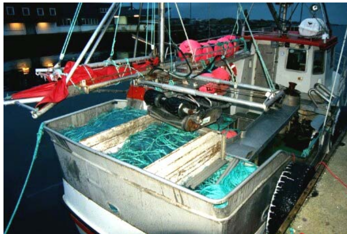
Figure 3: A modern Norwegian capture machine, 43 feet long, with about 150 monofilament nets and hydraulic equipment for net handling. Operated by two to three men. (Photo: J.P. Johnsen 2003.).
