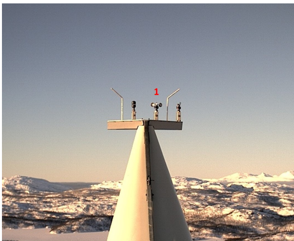
Figure 2.6: Anemometers and windvanes on the rear of the turbine nacelle. 1. KK-electronics anemometer.
