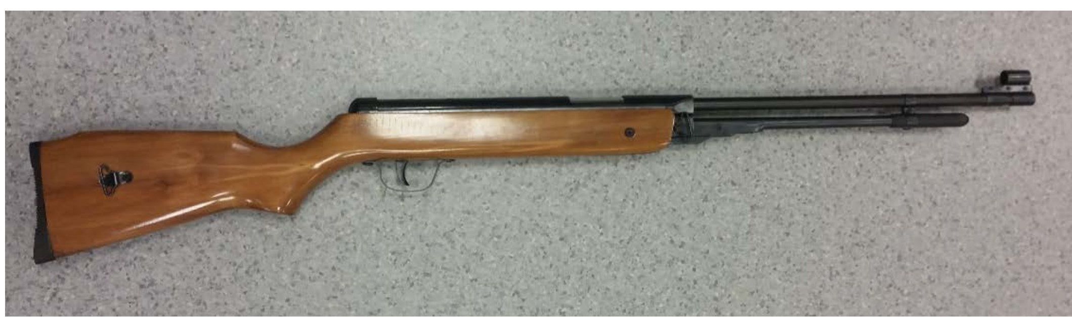
Air Rifle with 4.5mm caliber is using in the experiment
