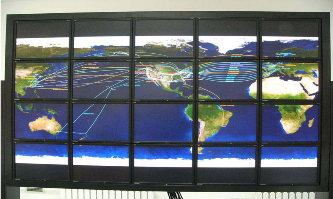
Figure 7 This is a snapshot of vnview image show application shown by a 4x5 monitor tiled display wall.
