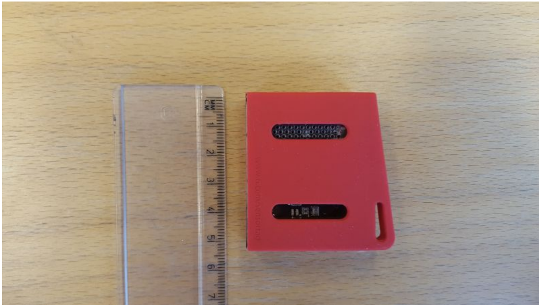
Figure 3.2: TI SimpleLink Multi-Standard SensorTag, CC2650 wireless MCU
