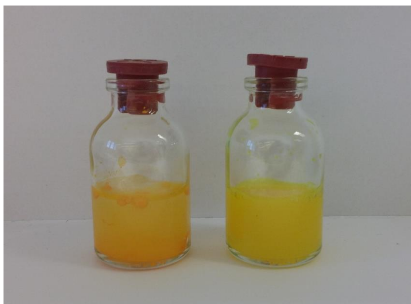
Figure 23: Bottle to the left contains curcumin in water. Bottle to the right contains curcumin entrapped in liposomal suspension in water.
