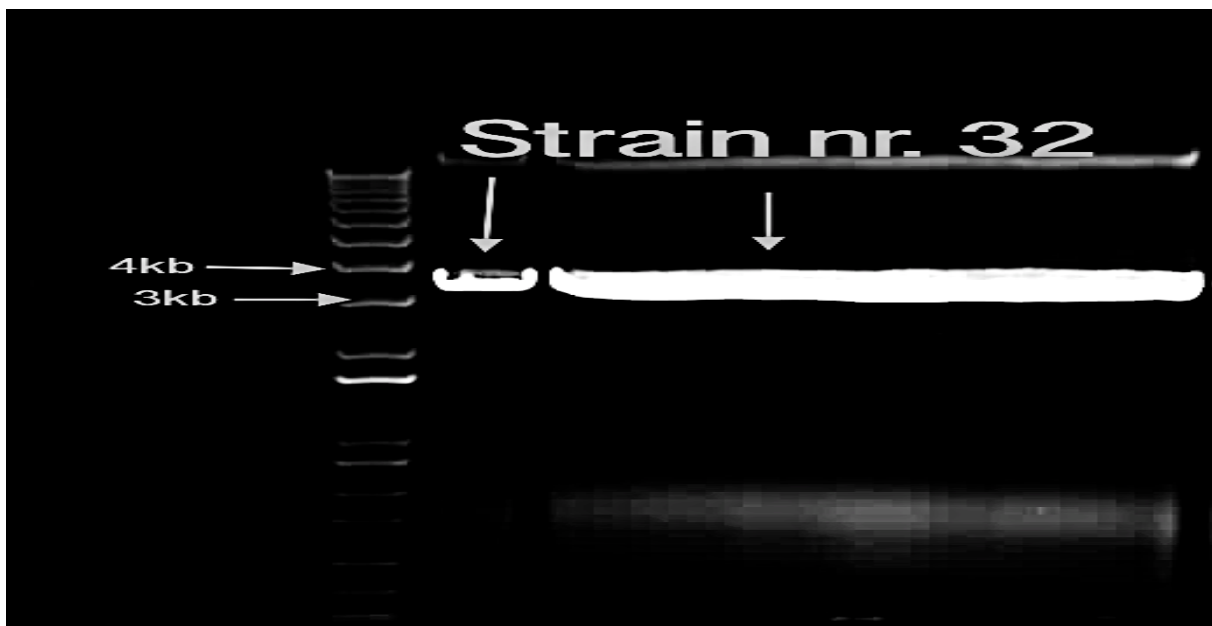
Figure 21: An image illustrated the PCR product of sdrD full length 3447 bp. Molecular weight standard (1Kb plus) used as marker.
