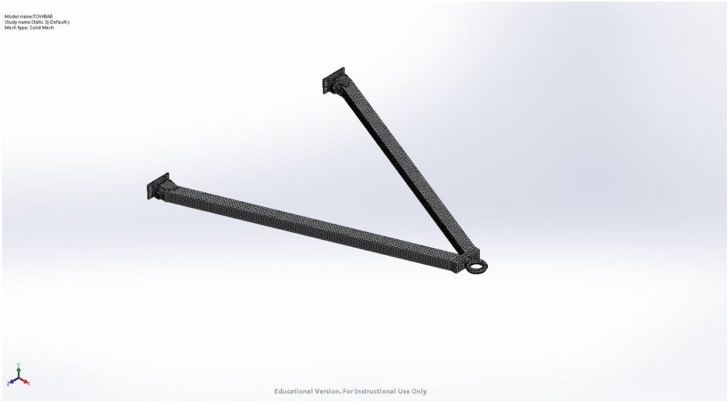
Figure 1: Model of the towbar, drawn in SolidWorks with applied meshing.
