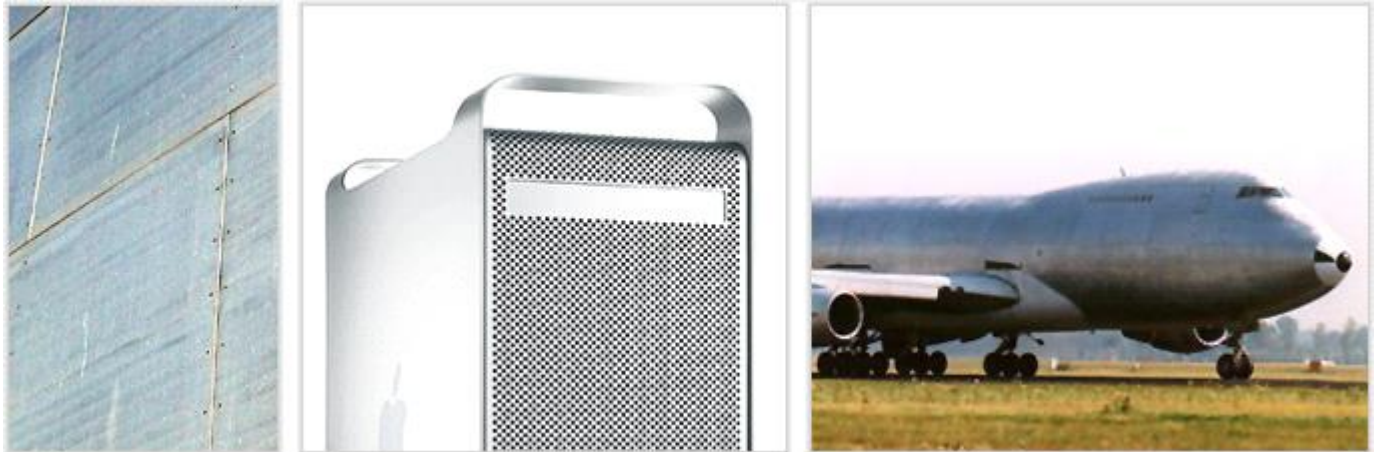
Figure 1: 1. A close-up of building cladding made from wrought aluminum alloy . © John Fernandez 2. Chassis of a personal computer. © Chris Lefteri 3. The 2000 and 7000 series age-hardening aluminum alloys are the backbone of the aerospace industry.
