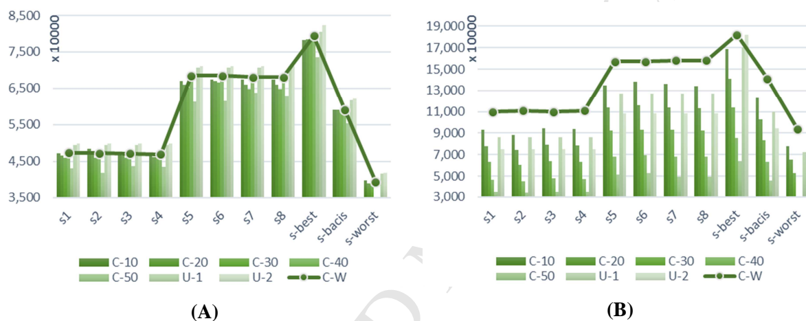
689 Figure.12 Comparison of the optimal solutions with respect to the changing parameters in the sensitivity analysis (results are 690 normalized by dividing by 10^4 ): (A) Carbon emissions from the facility operations; (B) Carbon emissions from the 691 transportation.
