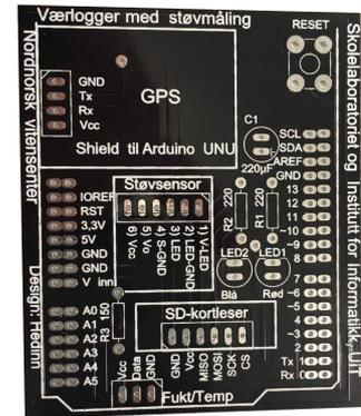
(b) The custom PCB Arduino shield.
