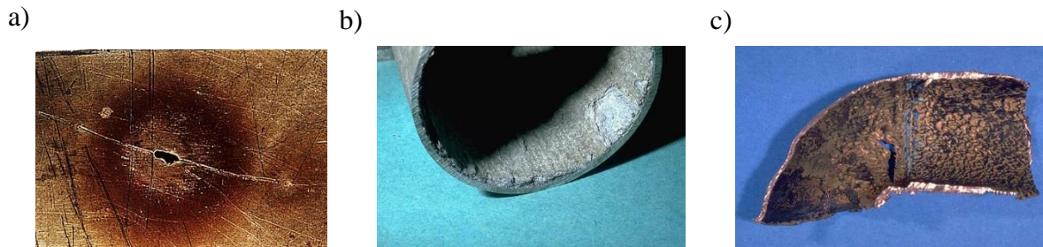
Figure 7 - Example of a) pitting corrosion; b) intergranular corrosion and c) erosion-corrosion (16)
