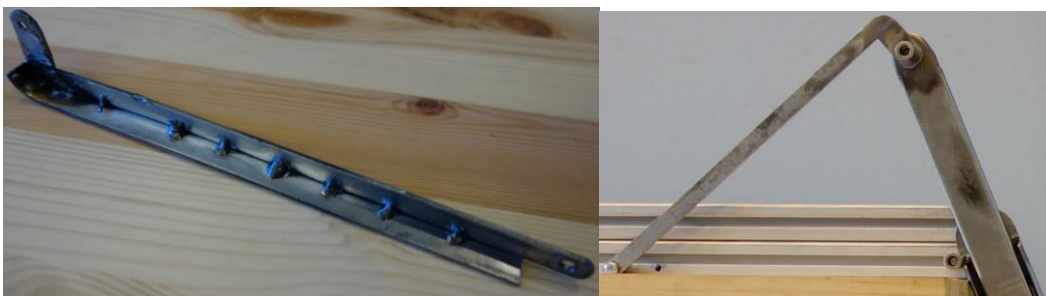
Figure 50 - Prototype IV. Details of the final iteration of the brace design [4].
