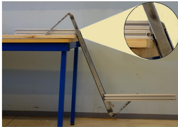
Figure 49 - Prototype IV. Magnified view of the motion stopper [4].
