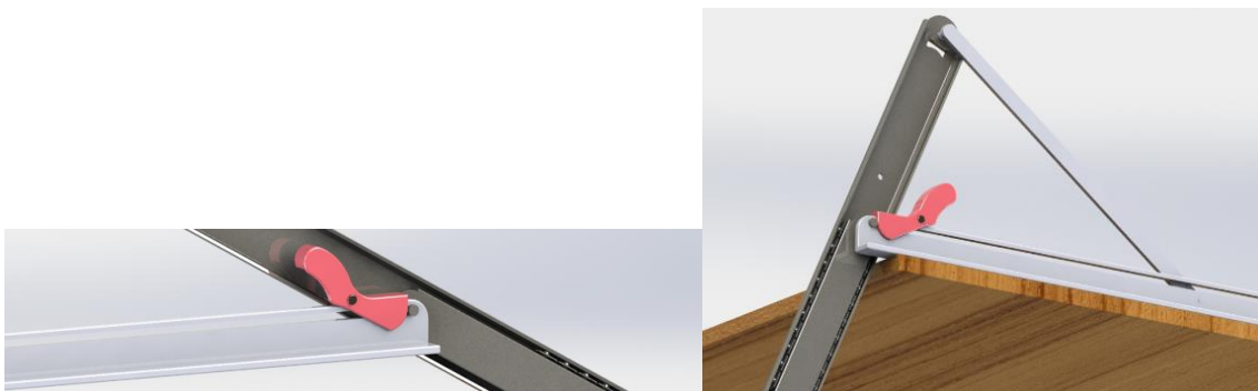
Figure 30 - Manual lever solution to prevent structural collapse [4].
