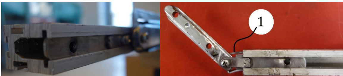
Figure 47 - Prototype III. Interaction between hinged slide element and aluminum profile [4].
