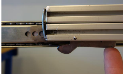
Figure 51 - Prototype IV. Manual motion stopper [4].
