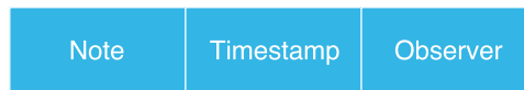
Figure 4.4: Timeout structure, the observer field is a local representation of a remote peer. There is no need to show byte indexes here since timeouts are not gossiped.
