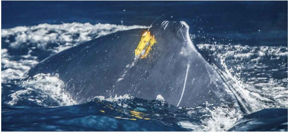
Figure 3. Time-depth recorder attached to a humpback whale under the dorsal fin. ©Audun Rikardsen
