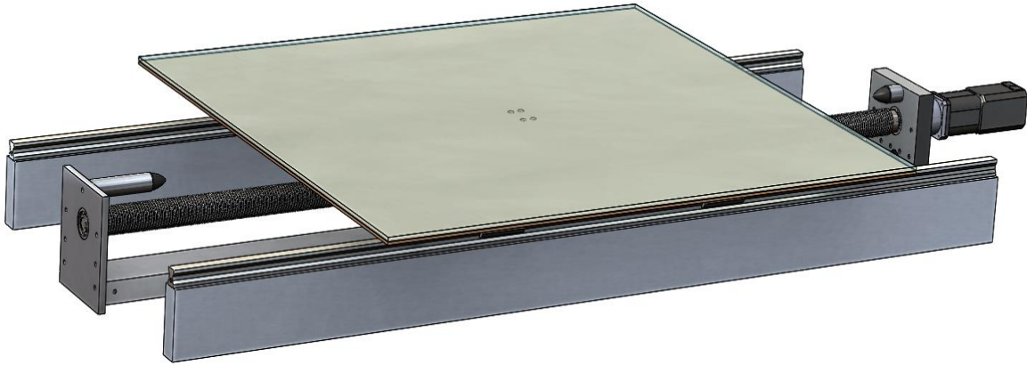
Figure 16. Y-axis and work table SolidWorks assembly
