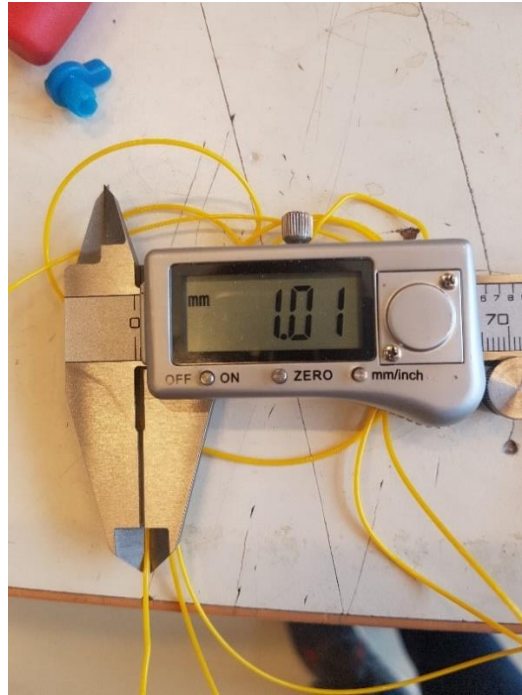
Figure 26. Measurement of the extruded filament
