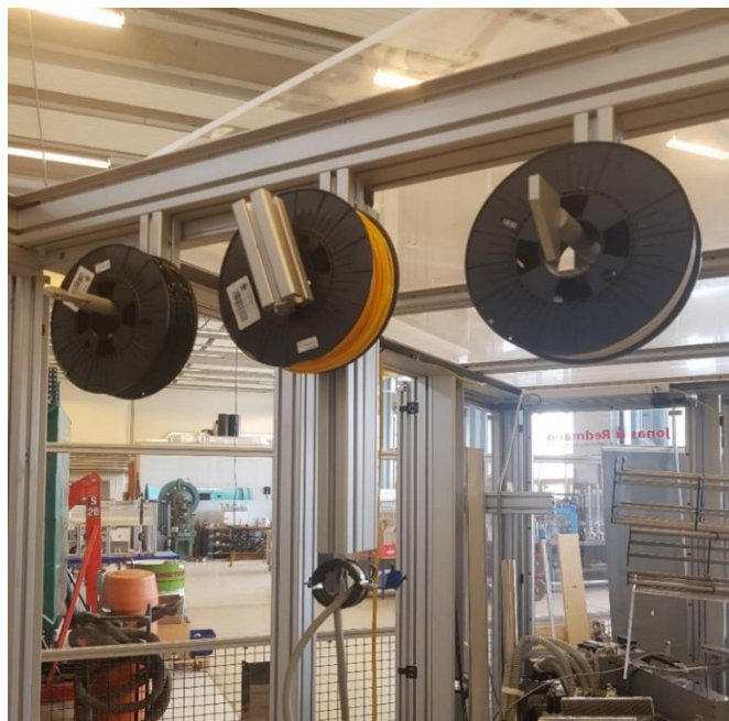
Figure 28. Filament rolls and wiring for the Duet
