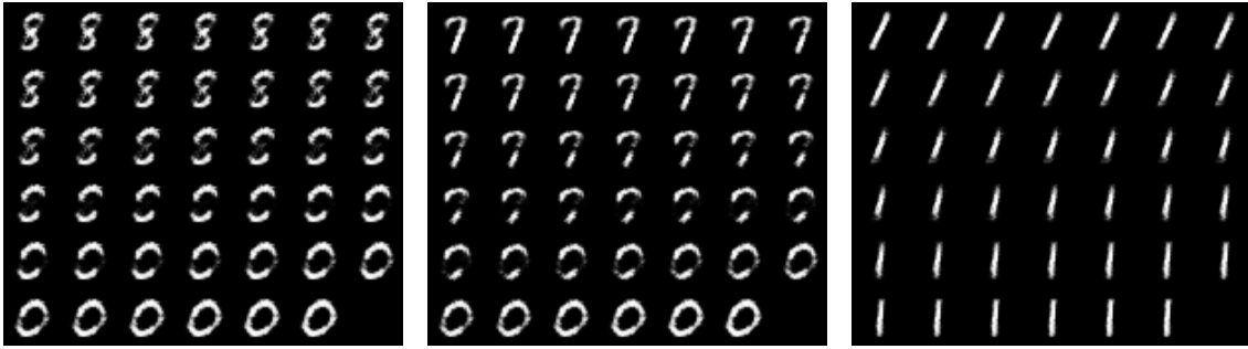
Figure 8: First and the last image of each panel show two k -means centroids in code space obtained on the MNIST dataset. Additional numbers are generated by “walking” on interpolated points between the two centroids.
