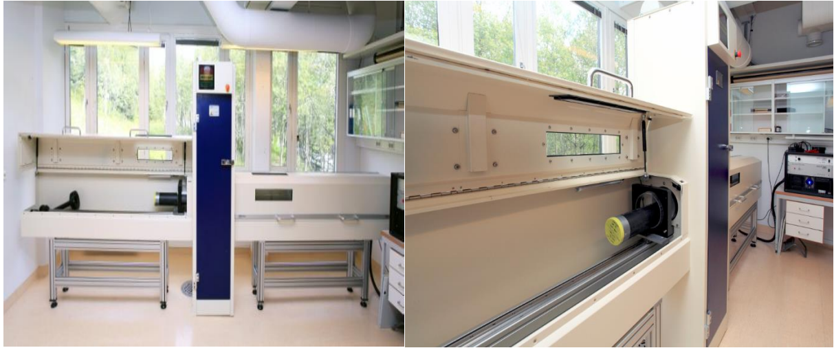
Fig. 3.2: Photos of the GEOTEK MSCL-XCT X-ray used in this study (adapted from UiT the Arctic University of Norway (2018a)).
