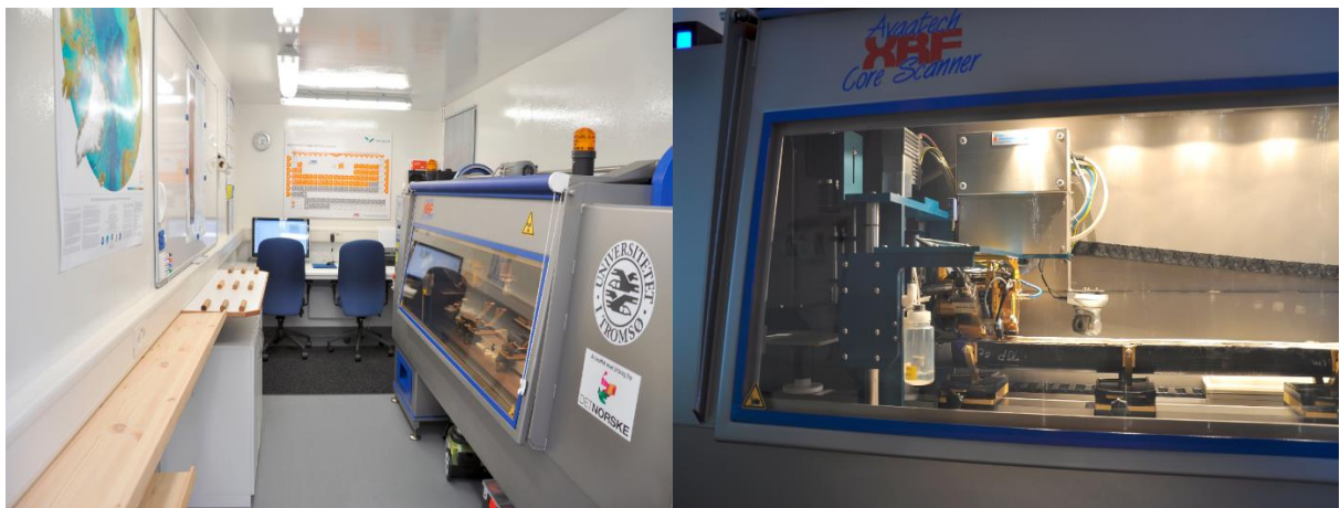
Fig. 3.3: Photos of the Avaatech XRF Core Scanner used in this study, which is placed in a container at UiT, The Arctic University of Norway (adapted from UiT the Arctic University of Norway (2018b)).
