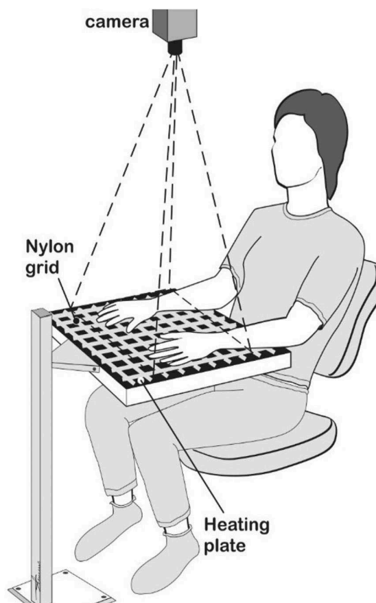
Figure 1. The set-up for dynamic infrared thermography (DIRT). Figure 1 reprinted with permission from Ina Isabella Høiland, the author of the master thesis at the UiT – The Arctic University of Norway; “The effect of oral uptake of nicotine on skin blood perfusion of the face and hands in snus users as determined by thermography” [18].
