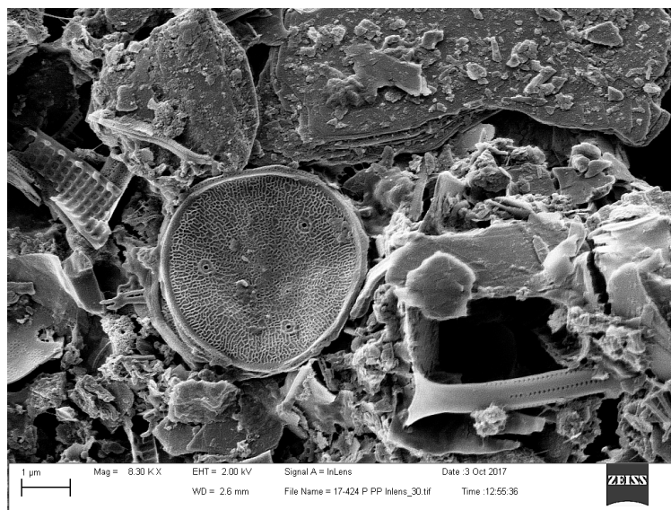
Figure 20. Organism of class Diatomea, possibly Bacillariophytina or Coscinodiscophytina , growing on a polypropylene pellet sample surface.
