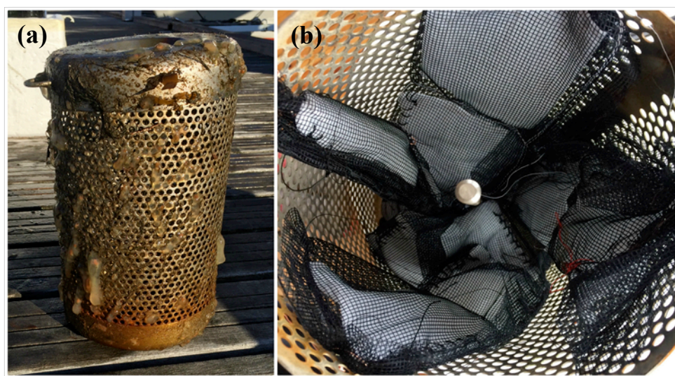
Figure 4. (a) Example cage used for submersion. (b) An inside view of the cage with the nylon sleeves and teabags containing pelletized polymers visible. (c) 2 g samples of microplastic pellets with paper clip for scale.
