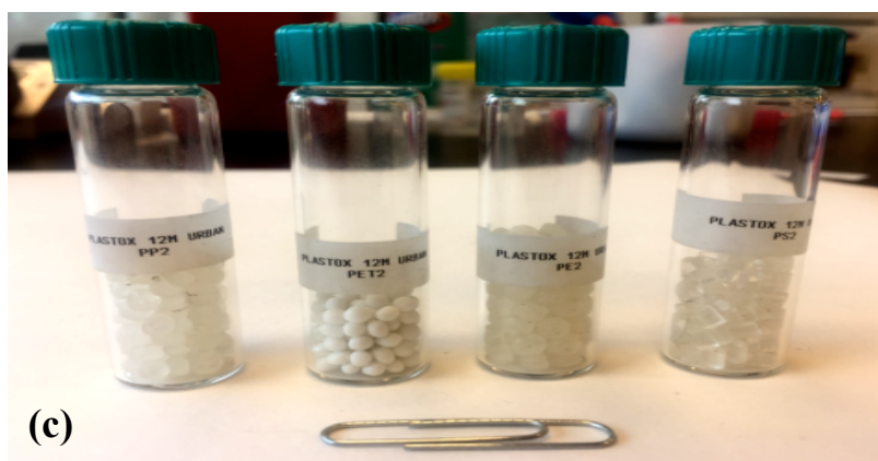
Figure 4. (a) Example cage used for submersion. (b) An inside view of the cage with the nylon sleeves and teabags containing pelletized polymers visible. (c) 2 g samples of microplastic pellets with paper clip for scale.
