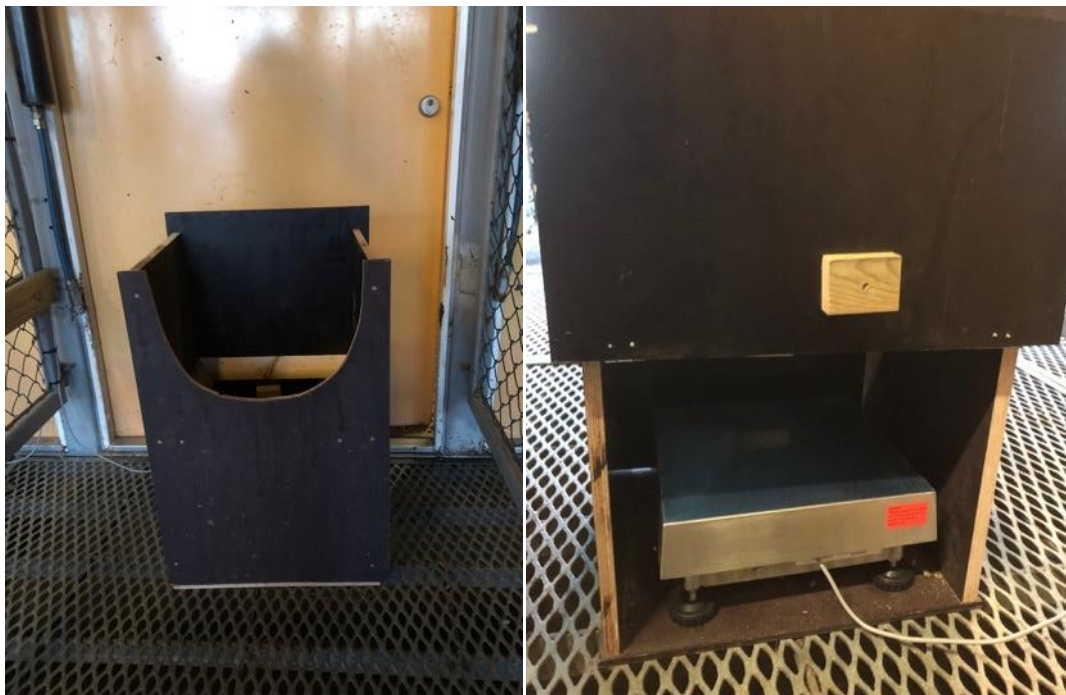
Figure 11. Front view (left) and back view (right) of the feeding boxes built to fit a weighing scale (as seen on the right picture).
