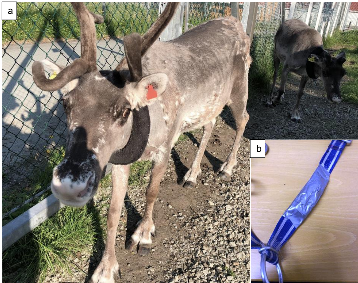
Figure 13. Soft collar cover and taping of actiwatch onto neck collar. (a) The furry collar covers prevented the collars from rubbing directly onto the skin, in particular when the animals were moulting from winter to summer coat. Both animals in the picture are members of the yearling group. (b) A collar with the actiwatch wrapped onto its outside with duct tape.
