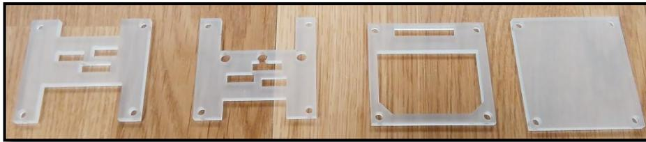
**Figure 27:** PCB insulating spacers manufactured using laser cutting machine
