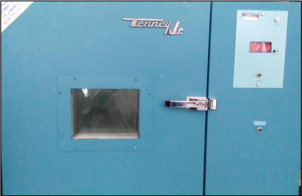
**Figure 49:** Cold Environmental Chamber (*Tenney Jr*)
