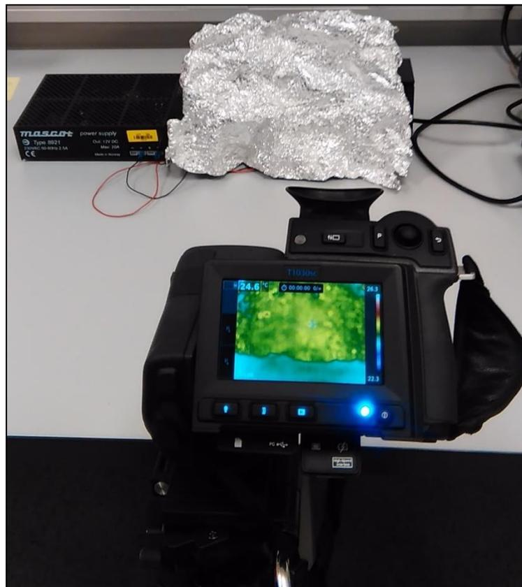
**Figure 51:** Setup for calculating reflected temperature at room conditions
