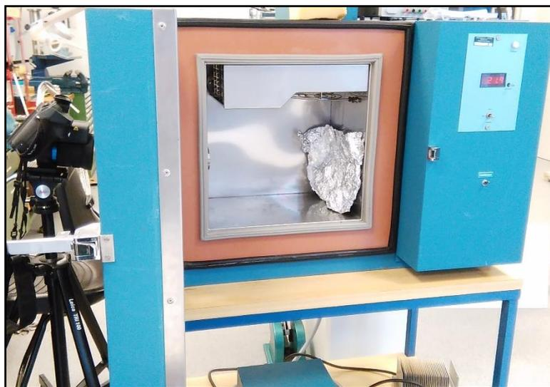
**Figure 53:** Setup for calculating reflected temperature in cold environmental conditions
