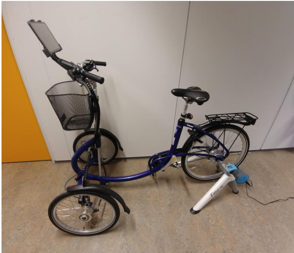
Figure 9 Tacx Smart Flow trainer with three-wheel bike and tablet on the handlebar.
