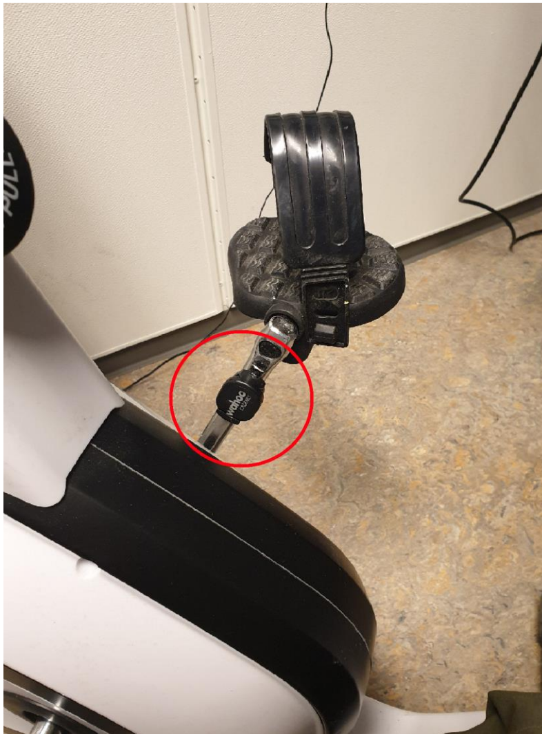
Figure 30 Cadence sensor mounted on the crank of the ergometer bike.
