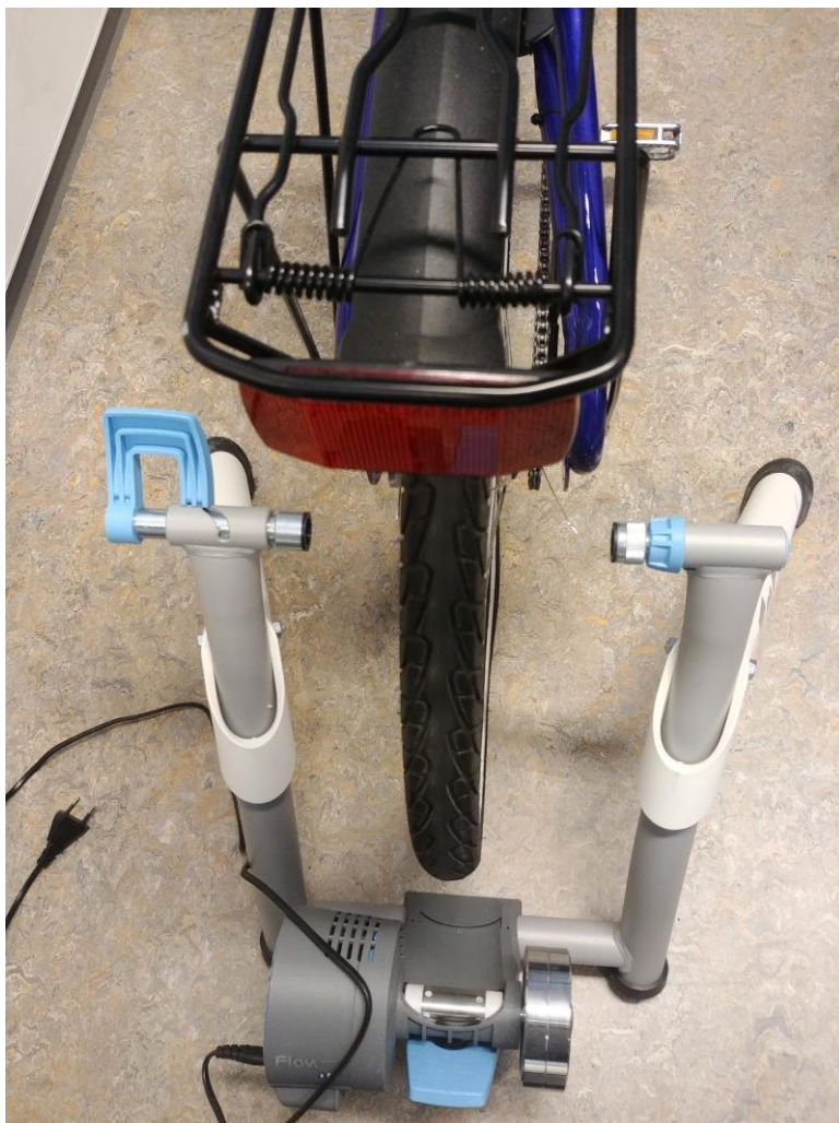
Figure 27A bike roller trainer before it is attached to the power wheel of the bike.
