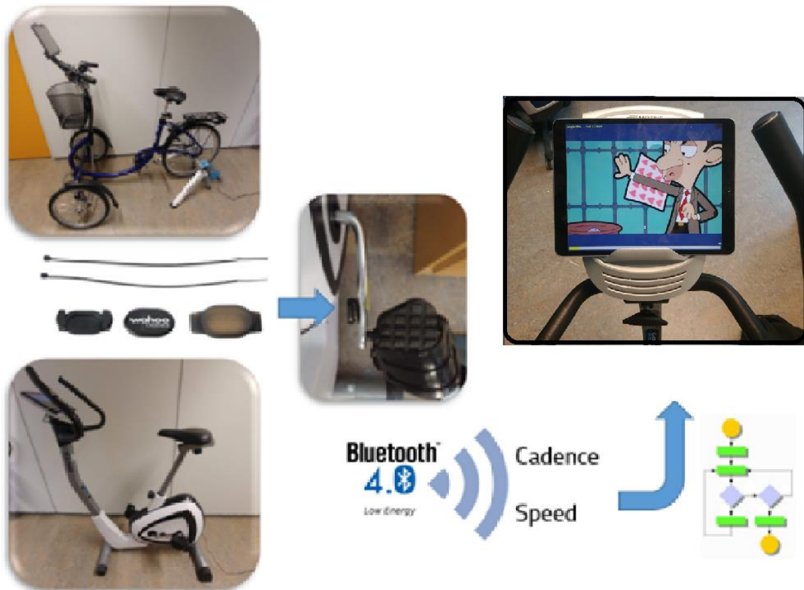
Figure 1 System outline, mount stationary bikes with sensors, and use activity data in an exergame customized for individuals with intellectual disabilities.
