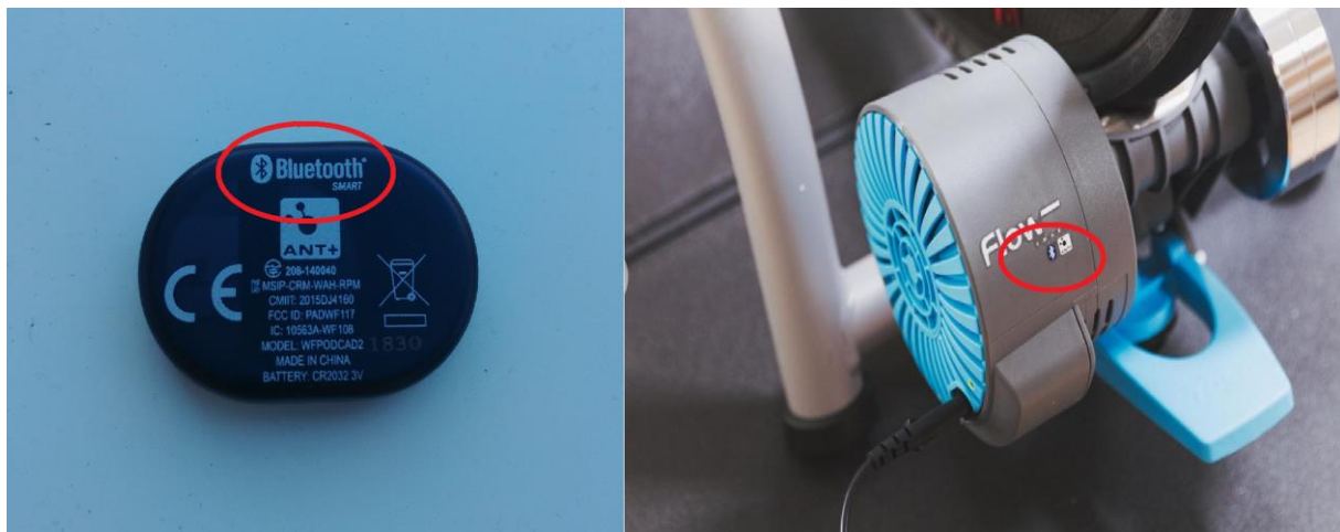
Figure 36 Bike sensors that support connection over Bluetooth Low Energy and measures either speed or cadence can be used in this system.
