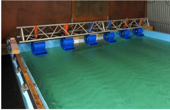
Figure 3. Water surface prior to the onset of freezing. (a) Arrangement of fans to create grease ice, and (b) separation of agitated section of the tank from quiescent area at the divider.
