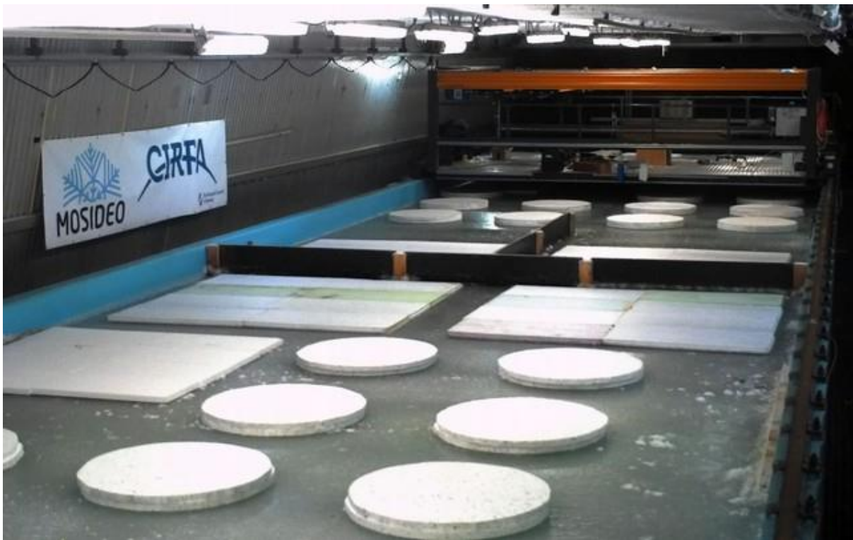
Figure 4. Surface insulation to create an under-ice profile.
