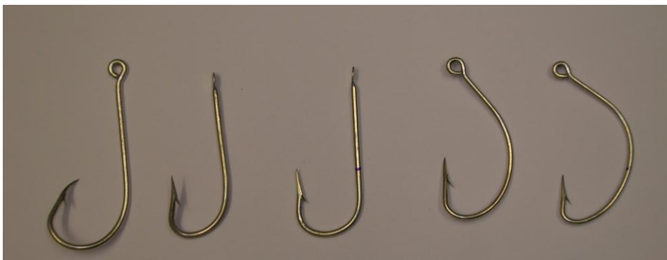
Fig. 15: The hooks tested. From the left EZ-baiter (B), Kirby (Z), Round Bend Sea (D), Wide Gap (C), Wide Gap Eyed (A).
