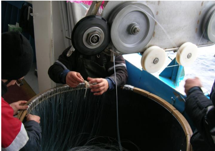
Fig. 10: The first fisherman operating with the winch (right) gives the snoods to the the second and third fisherman (left).
