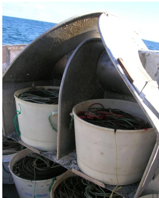
Fig. 14: Double line chutes utilized by Norwegian coastal longline boats.
