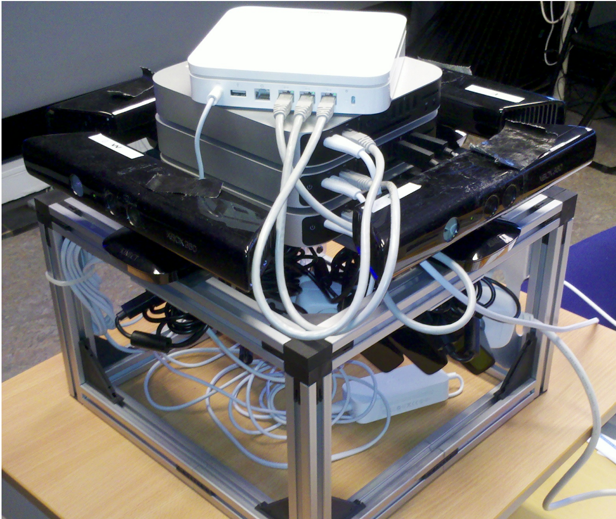
Figure 2.5: The four 3D Kinect camera rig used on each stage for almost 360-degree coverage.
