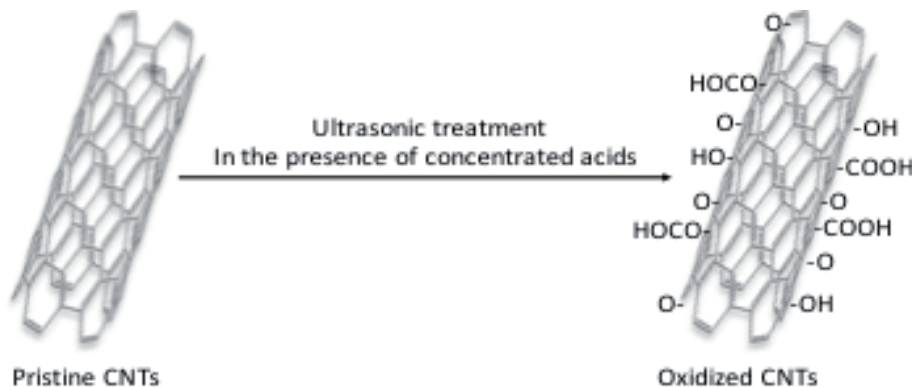
Figure 3. Oxidation process of CNTs under harsh conditions.
