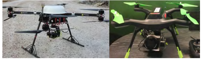
FIGURE 2. Our custom-built full-scale UAV (left) for large-scale inspections and back pack UAV (right) for small-scale inspections.
