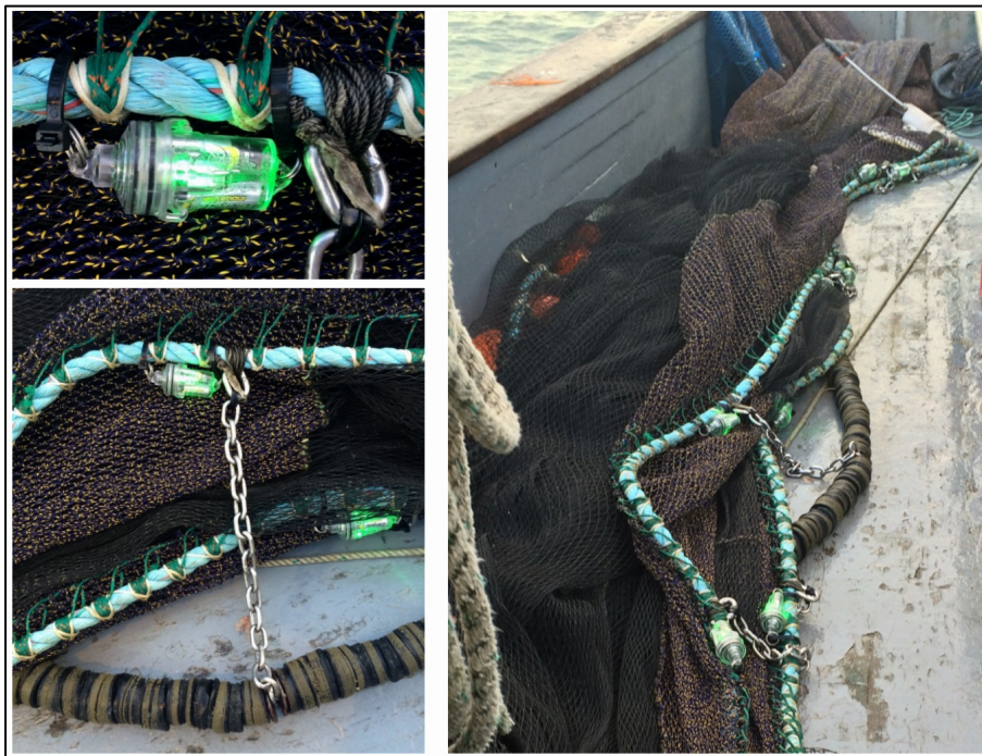
Figure 8. Images of artificial illumination placed along the fishing line of an ocean shrimp trawl as a technique to reduce fish bycatch. Source: Hannah et al. (2015).
