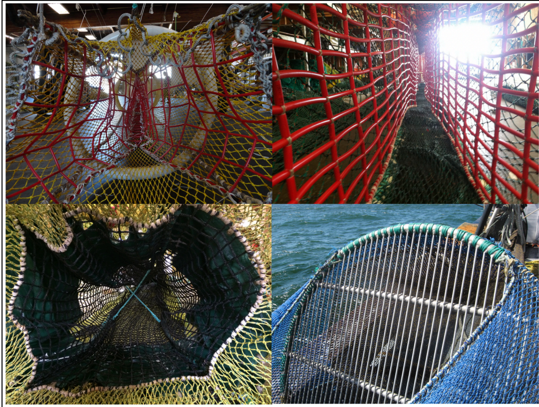
Figure 4. Example of sorting grid BRDs designed to reduce bycatch of Pacific halibut (top left image) and roundfishes (top right image) in the West Coast groundfish bottom trawl fishery, rockfishes in the Pacific hake fishery (bottom left image), and fish in the ocean shrimp fishery (bottom right image).
