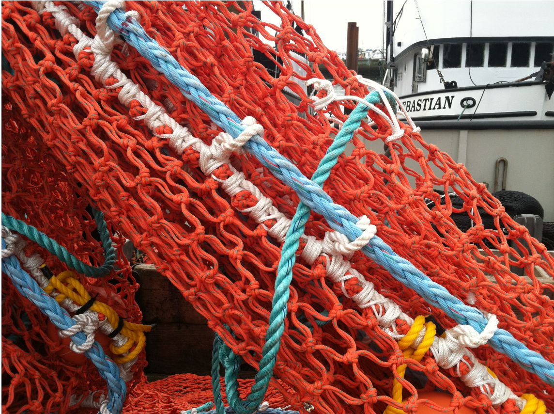
Figure 15. Image of a T90 mesh codend manufactured for a U.S. West Coast groundfish bottom trawl vessel.
