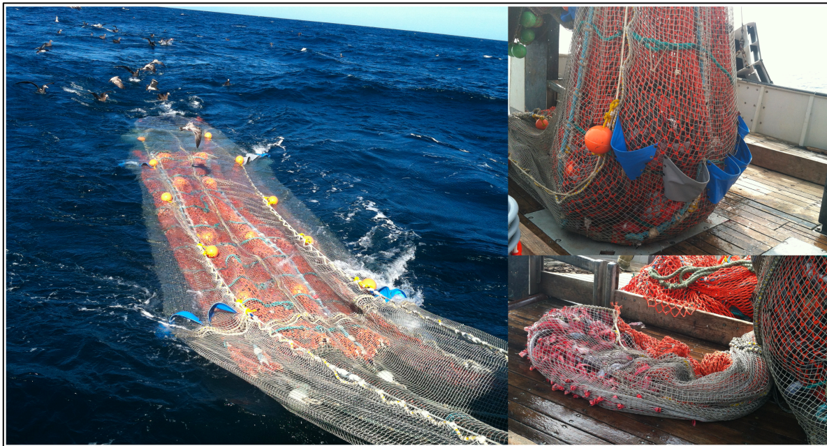
Figure 9. Example images from a tow using the covered-codend sampling technique. Covered-codend during haulback at the sea surface (left image); catch retained in the trawl codend (top right image); catch that escaped out the trawl codend and was retained in the cover (bottom right image).
