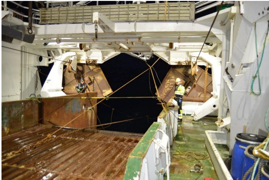
Picture 2: Crew member on the Port and Starboard Trawl door positions under hauling of the trawl (Roger B. Larsen, UiT – The Arctic University of Norway).
