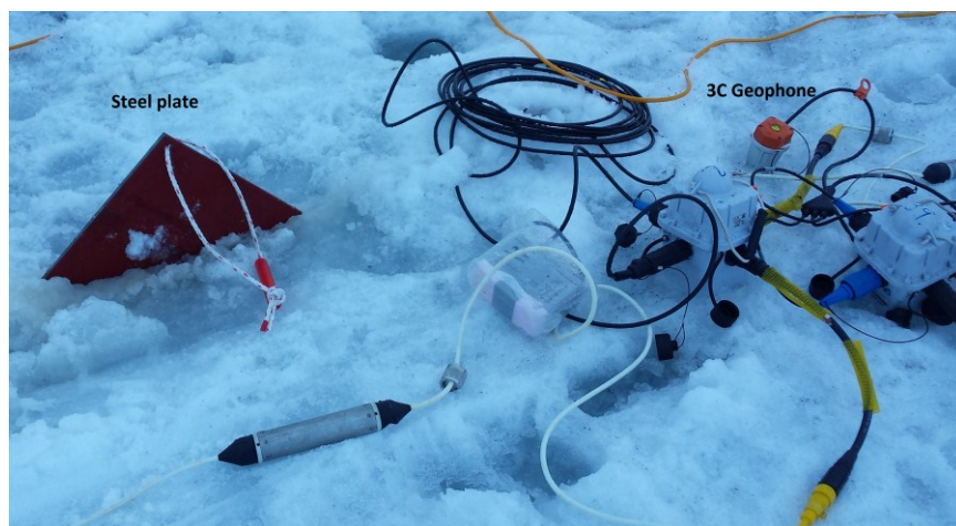
Figure 4. a) Steel plate frozen into the sea ice used as shear wave source. b) Data from experiment E1 in Table 1 showing 3-component recordings from a sledgehammer blow transverse to the line. In the upper figure showing the three components at 100 m offset, the components have the same scale, while in the two lower figures the traces have been scaled individually (there are four dead traces on each of the lower figures due to improper coupling of geophones in the setup). The extensional Lamb wave is seen only on the radial (R) component while the much stronger shear-horizontal (SH) wave is seen on both the transverse (T) and radial component. The SH waves on the R component might indicate a small error in the orientation of the 3C geophones.
