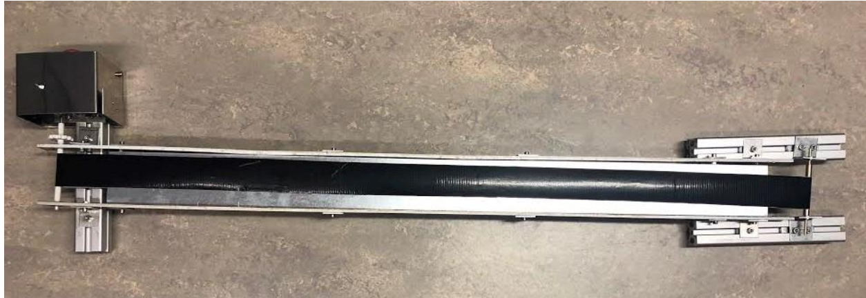
Figure 57: Constructed Conveyor Belt
