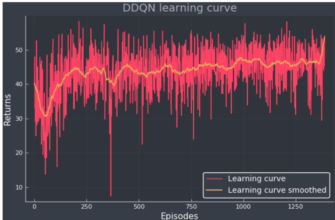
**Figure 4.9:** The DDQN learning curve, displaying how the return evolves with training episodes. The red curve is the original return data and the orange curve is a smoothed version, which is easier to interpret.
