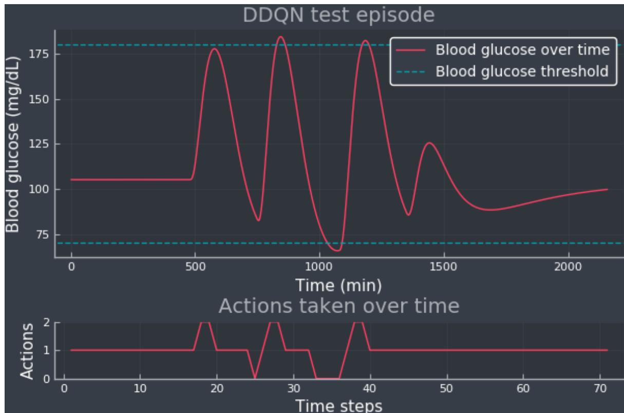
**Figure 4.7:** A DDQN test episode showing the BG curve (upper panel) and the actions selected over time (lower panel). The blue dotted lines indicate the normoglycemic range and it is fixed at 70-180 mg/dL.
