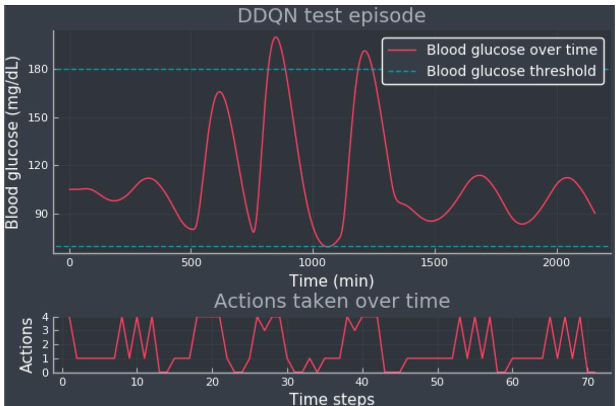
**Figure 4.32:** A DDQN test episode showing the BG curve (upper panel) and the actions selected over time (lower panel). The blue dotted lines indicate the normoglycemic range and it is fixed at 70-180 mg/dL.
