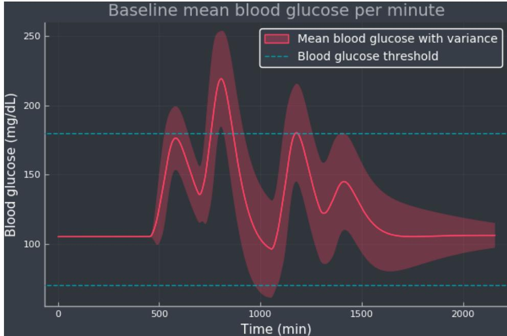
**Figure 4.3:** A baseline BG curve with meal disturbances using only the optimal basal rate  $b^* = 6.43$  mU/min as the selected action. The curve is the mean BG per minute with confidence bands (shaded red area), representing the standard deviation, simulated for 100 episodes and with a 10% probability to skip meal boluses. The blue dotted lines indicate the normoglycemic range and it is fixed at 70-180 mg/dL.
