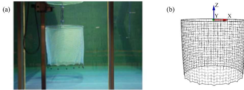
Fig. 20. The fish cage in still water shown from the side: (a) the physical fish cage model, (b) the numerical fish cage model. The numerical model is subjected to the flow along the x-axis.
