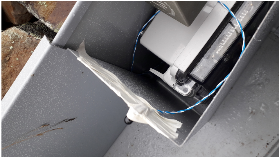
Figure 8.1: This picture show how the IR transistor is secured in the camera trap (Photo: Michael J. Murphy)
