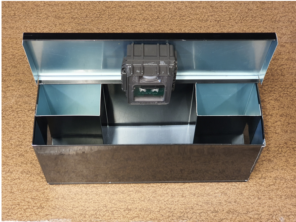
Figure 2.1: A dimensional accurate camera trap prototype we have in our office. Color and lid mechanism has changed in deployed camera traps. (Photo: Øystein Tveito)
