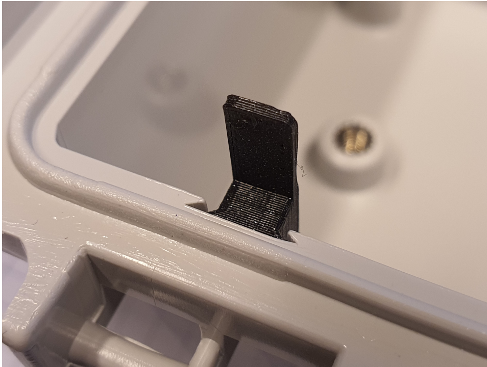
Figure 9.1: Photo of the spacer slotted into the sensor node enclosure (Photo: Øystein Tveito)
