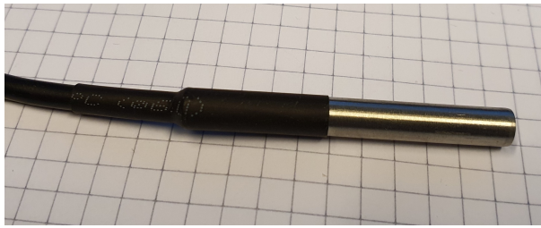
Figure 7.5: DS18B20 temperature sensor with waterproof housing (Photo: Øystein Tveito)
