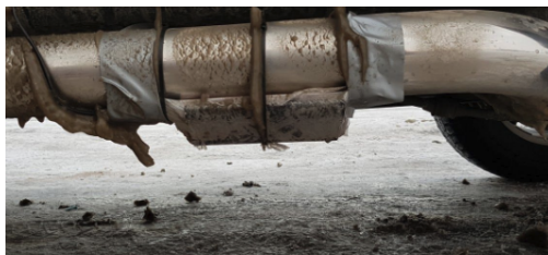
Figure 15.2: Placement of the sensors on the vehicle. Top image by OpenClipart-Vectors from Pixabay.
