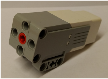
Figure 10.7: The EV3 Medium Motor sensor.
