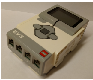
Figure 10.8: The EV3 intelligent brick.
