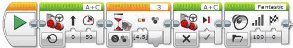
Figure 10.4: An EV3 software program that makes the robot drive forward until the color red or yellow is seen. Then the robot stops and shouts "Fantastic".
