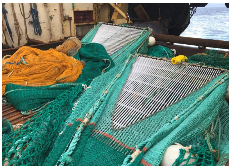
Figure 10: The grids used in the sea trials (Photo: Hermann Pettersen).
