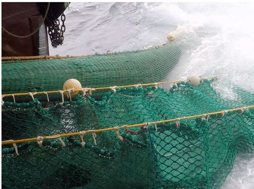
Figure 6: Two codends, (lower) with 30% shortened lastridges, (upper) no shortening of the lastridges.
