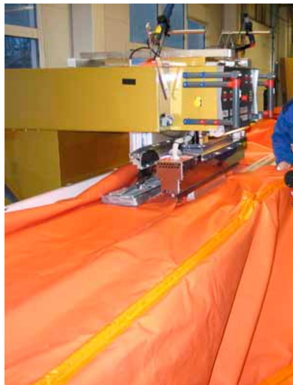
Figur 3.6. Plastsveisemaskin for store presenninger.
