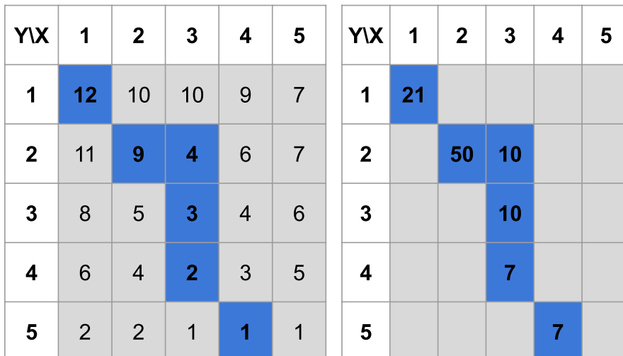
FIGURE 2 (a) Schematic raster representation of a stream (blue cells) imposed on a digital elevation model (DEM) and (b) resulting slope measures in degree * 100 computed as elevation difference between neighbouring pixels along the stream. Slope of grid cell x_1y_1 and next cell in the stream x_2y_2 is computed using: \text{round}(\text{degrees}(\text{atan}((12 - 9)/\sqrt{(10^2 + 10^2)})) * 100)
