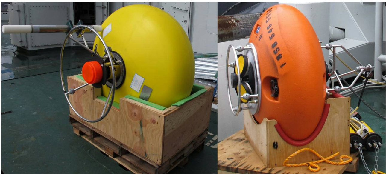
Figure 15.1. Left: a Simrad WBAT echosounder mooring ready for deployment. The orange disc is the acoustic transducer, the yellow cylinder (mostly obscured) is the WBAT echosounder, the yellow ellipsoid the flotation, and the white/silver tube an ARGOS tracker. Right: A Nortek Signature100 echosounder mooring ready for deployment. The echosounder transducer is the black disk to the left, and the yellow discs the ADCP transducers.
