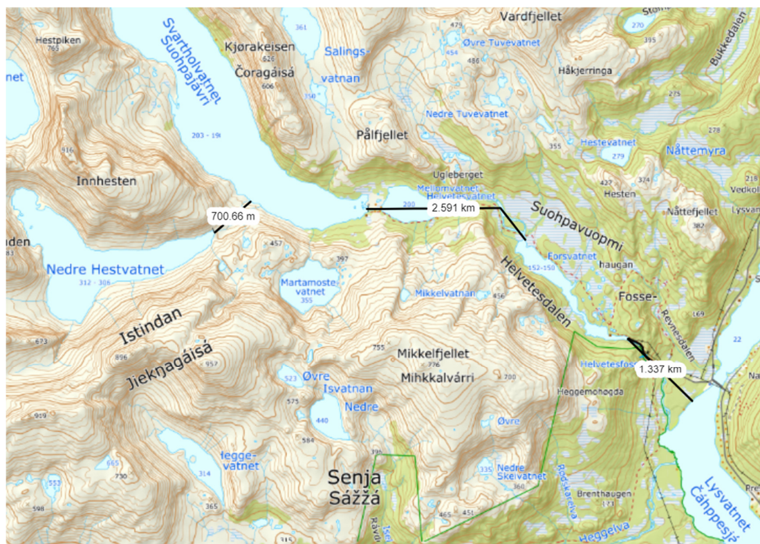
Figure 5-8 Three alternative layouts for using Lysbotn power plant as PHEs illustrated by black lines. The lines are giving the horizontal distance, and the height of the lakes are given by blue values (Norgeskart, 2019).
