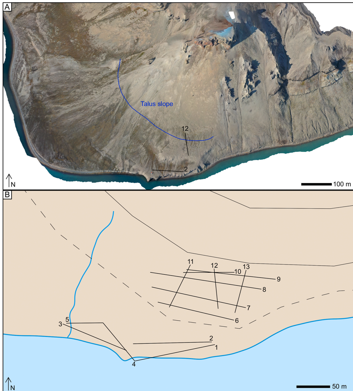
Fig. 5. GPR survey profile locations. A: Overview DOM showing the Talus slope and locations of key GPR profiles 2 and 12. B: Map of Rudmosepynten showing the locations of the GPR profiles 1–13 used for the integration and interpretation in this paper. Map from: Norwegian Polar Institute (2014) . (For interpretation of the references to color in this figure legend, the reader is referred to the Web version of this article.)
