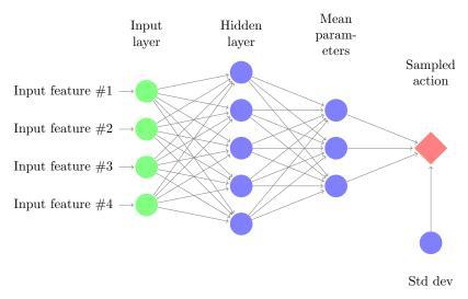
**Figure 2.** Neural network policy parameterization. The neural net maps the state, in this case a 4 dimensional space, to the mean,  $\mu$ , of the Gaussian policy. The output is then a sample from the Gaussian policy  $\mathcal{N}(\mu, \sigma^2)$ . The  $\sigma$  parameter is in this work the output from a neural network.
