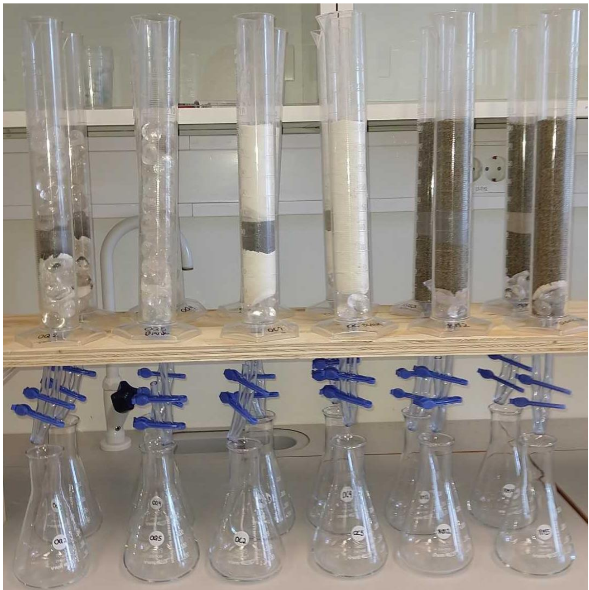
Figure 15: Kinetic column test setup. Every column and flask marked with respective conditions OC (1, 2, 3, 4), OQ (1, 2, 3, 4) and RM (1, 2, 3, 4). Picture from the lab. 3.9.2018 by Birgitte Fagerheim.
